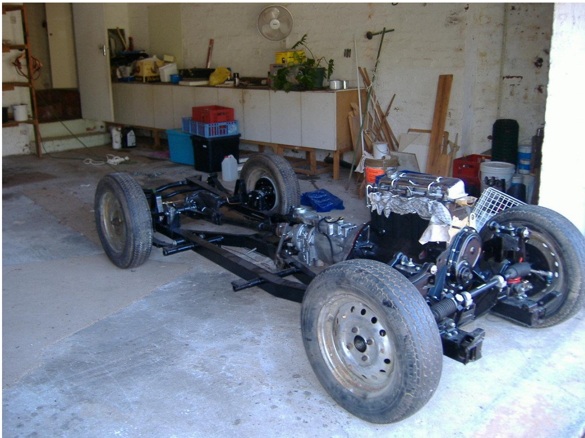
THE TR4 CHASSIS HAS MUCH IN COMMON WITH THE EARLIER SIDESCREENS
