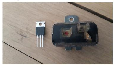
uppermost when sorting out the wiring in order to prevent irreparable damage to the stabilizer. With the black box uppermost the left prong is connected to an "ignition on" power supply, the middle prong goes to earth and the right hand prong directs the 10v power supply to the 2 instruments. I soldered three wires in place and
