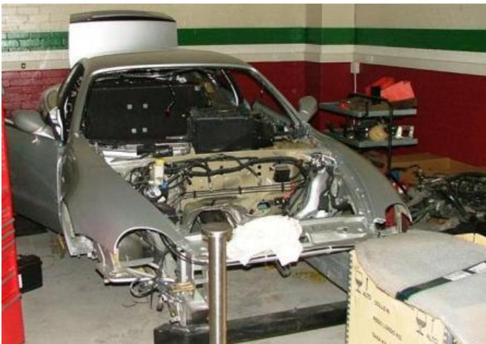
In one of the corners of the storage facility, we found a Maserati that had recently been modified by its owner, while he was attempting to cross a kerb at high speed. The Maserati's suspension had been damaged extensively and was in the process of being replaced.
