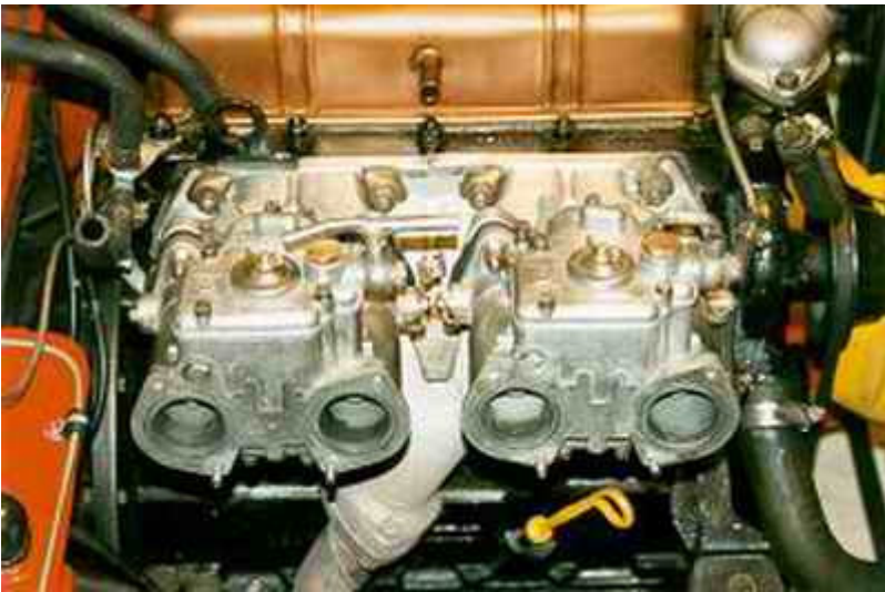
THE FINAL SETUP SHOWING THE NEW THROTTLE LINKAGE
