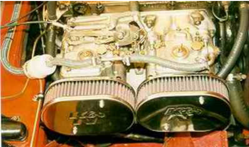
THE FINAL SETUP SHOWING THE NEW THROTTLE LINKAGE
